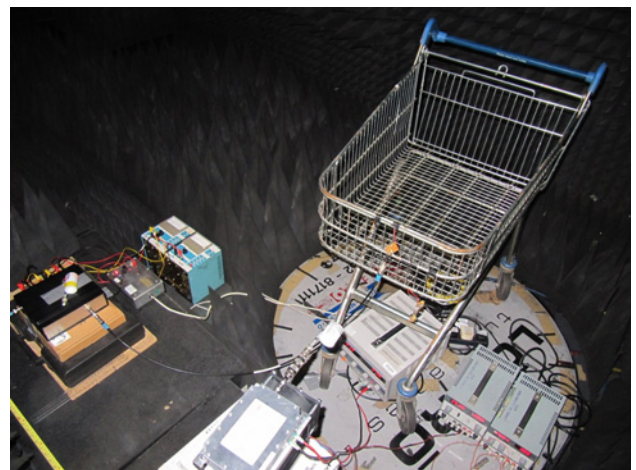
Fig. 11 Shopping trolley eavesdropping arrangement
