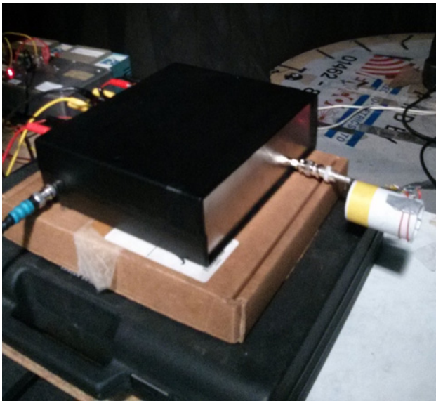
Fig. 8 Receiver circuit and eavesdropping antenna
