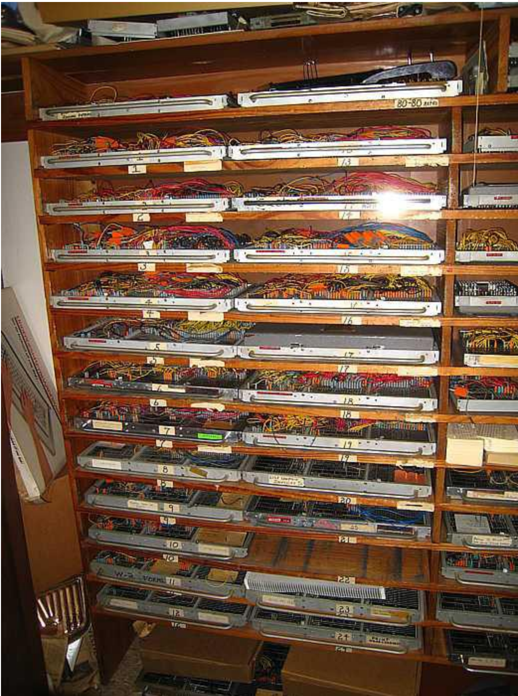
Sparkler Filters' collection of IBM 402 programs on IBM plugboards. (Photo Courtesy Ed Thelen / IBM 1401 Group)
