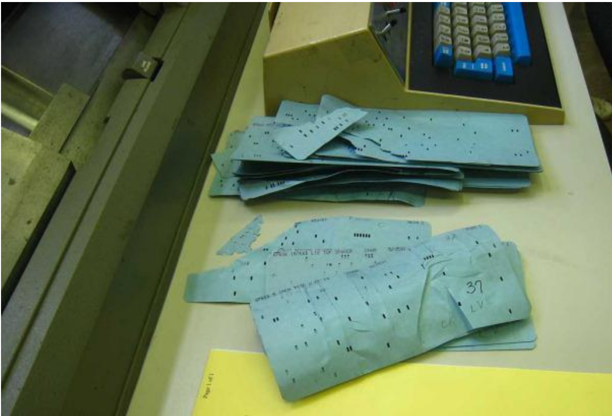
The punched cards used in the 402, with some mangled cards from a recently cleared jam in the card reader. The cards sit on the IBM 029 key-punch machine. (Photo Courtesy Ed Thelen / IBM 1401 Group)
