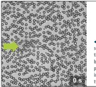
Optical microscope images separated by 6.63 s showing the formation of chains between only the large particles starting from an initially random mixture of two particles sizes.
