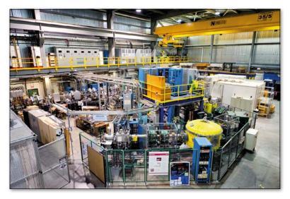
▲ FIG. 5: DRAGON, an example of recoil mass separator for the study of nuclear reactions of astrophysical interest, located in the ISAC facility at TRIUMF (Vancouver). Image courtesy of Steven Oates. Li production and on the origin of R Cor Bor stars (a variety of hydrogen-deficient stars with high carbon abundances);
