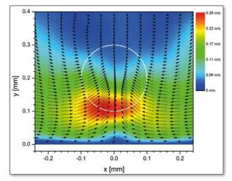
▲ Simulated velocity field of the microfilament in the vicinity of the dielectric wall after the train of 150 localised breakdowns.
