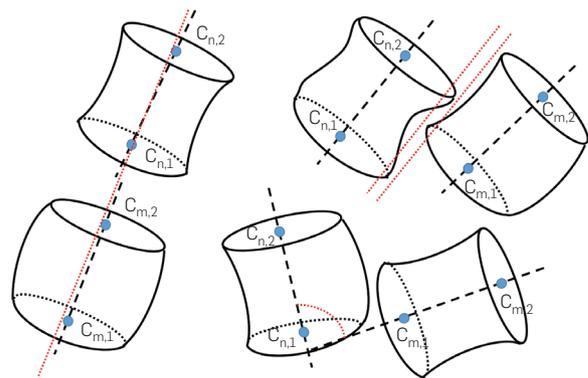
**Figure 5. Determining coordinates  $C_{i,j}$  for axis endpoints of a cuboid from the depth value  $z_i$  of the reference point  $R_i$ .**
